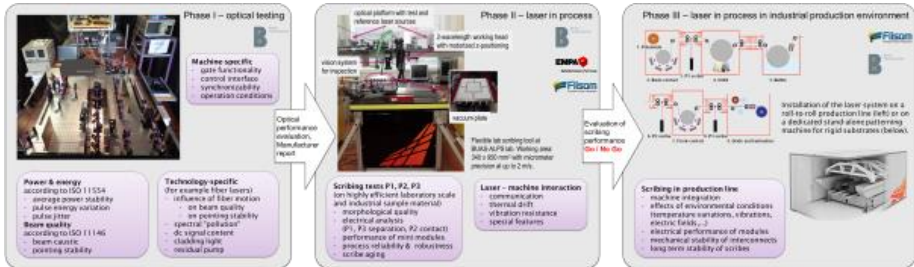
Schematic representation of the 3-stage assessment process in CIGS solar cell scribing
