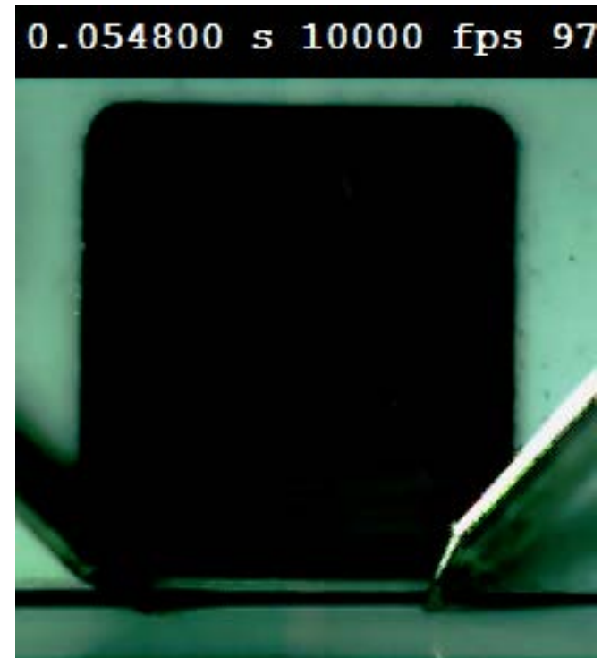
high-speed recording of a reacting Nanofoil ® , total time: 2.5 milliseconds
