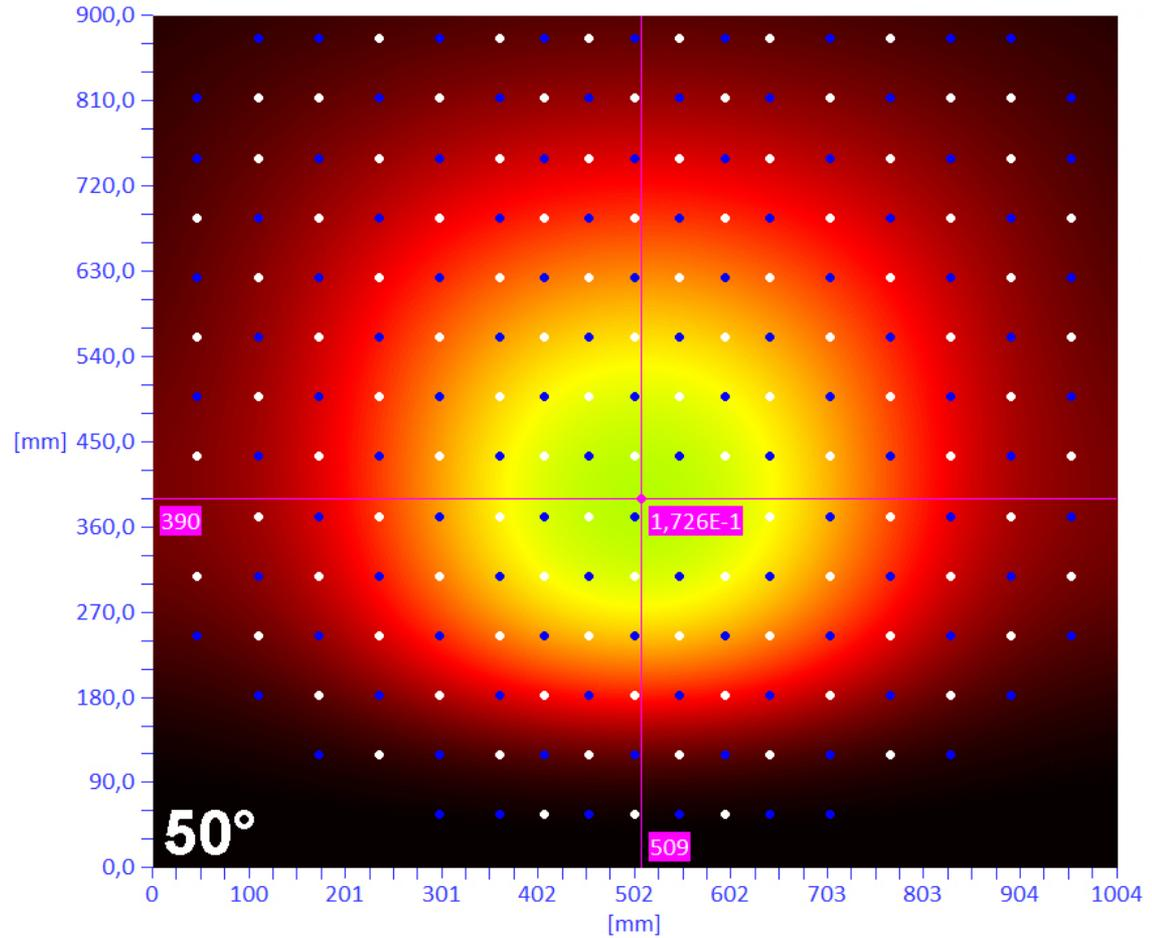
Uniformity of  $\text{TiO}_2$  layers  $\varnothing 430\text{mm}$  without shaping masks
