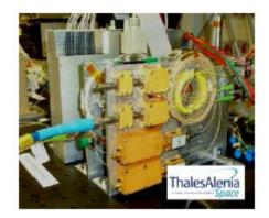
Figure 4-22: Photonic Router/Wavelength Selective Switch
