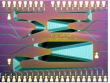
Figure 4-30: Photon First (NL) Microphotonic FBG Interrogator based on InP Photonic Integrated Chip.
