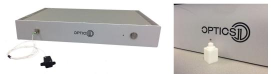
Figure 4-32: Optics 1 optical sensor interrogator (left) and 3-axis accelerometer prototype (right).
